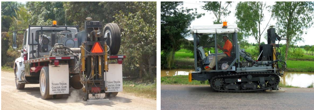
Figure 2 Truck mounted accelerated weight drop system (left), and Morooka mounted accelerated weight drop system (right). The Morooka's manoeuvrability makes it better for maintaining acquisition production rates along narrow tracks and over rough terrain.
